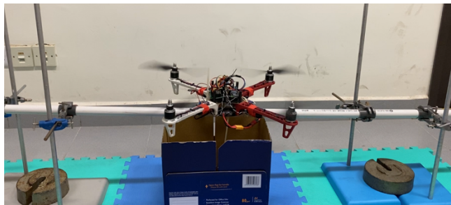
Figure 3: Quadcopter secured to a rod allowing for rotation about a single axis
