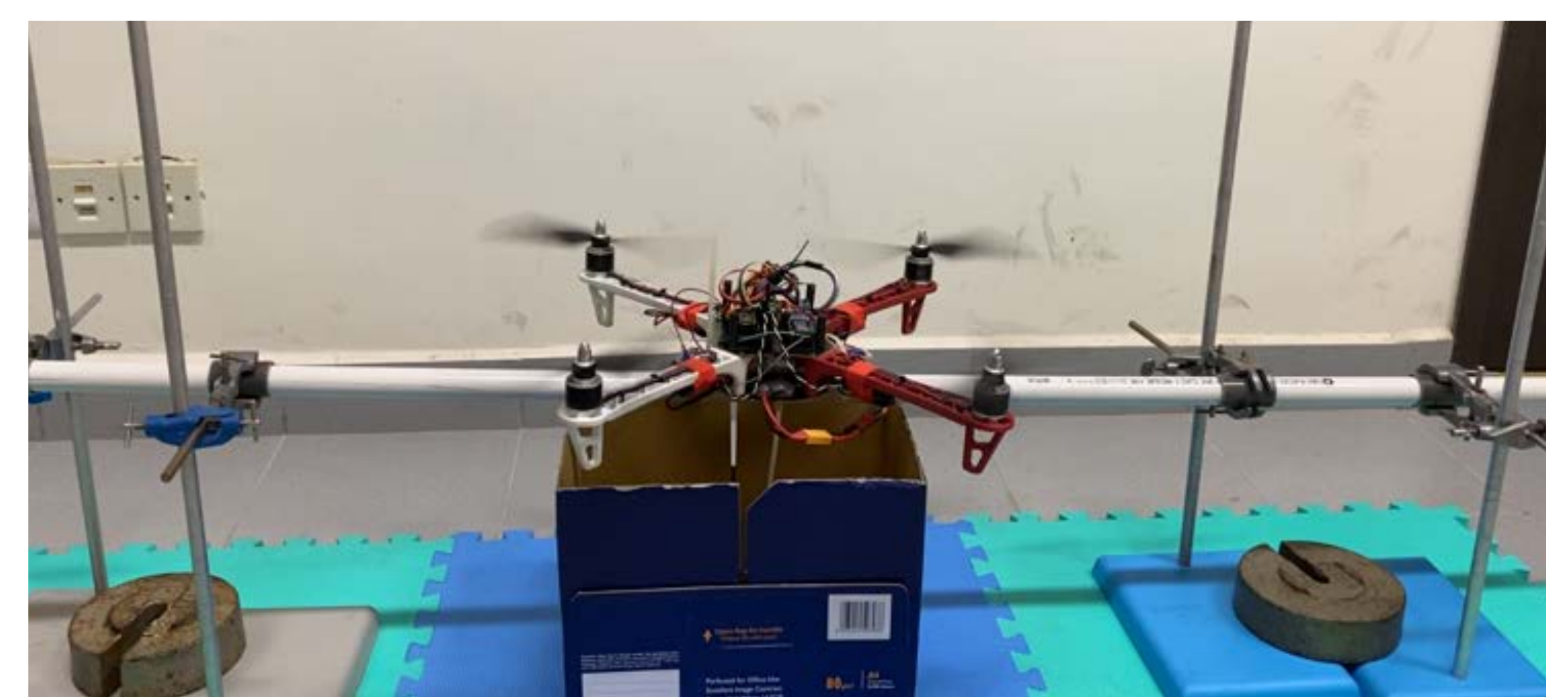
Figure 5: Quadcopter secured to a rod allowing for rotation about a single axis
